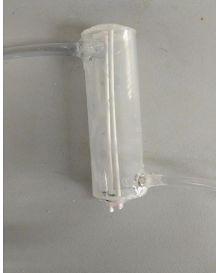
Figure 2. Alumina hollow fiber membrane module B (with two membranes).
