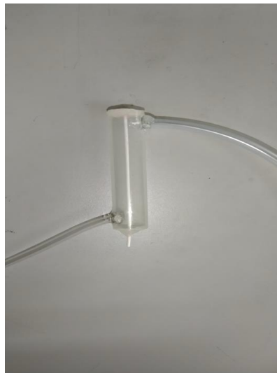
Figure 1. Alumina hollow fiber membrane module A: A single membrane.
