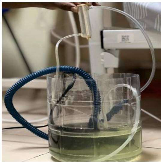
Figure 4. Setup for alumina hollow fiber membrane module experiment.
