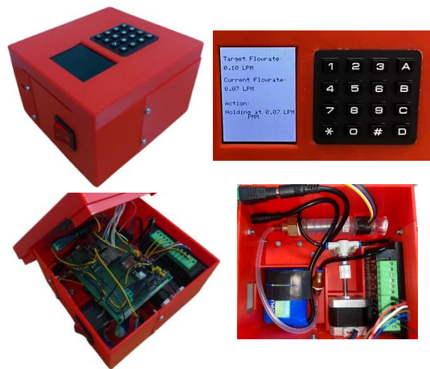
Figure 5. Printed device casing; component assembly in the casing and TFT and keypad user interface.
