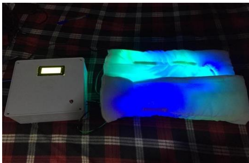
Figure 6. Developed low-cost phototherapy neonatal biliblanket.
